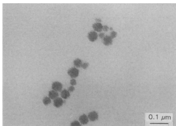
Figure 2 Transmission electron micrograph picture of tin oxide particles prepared by grinding technique.
